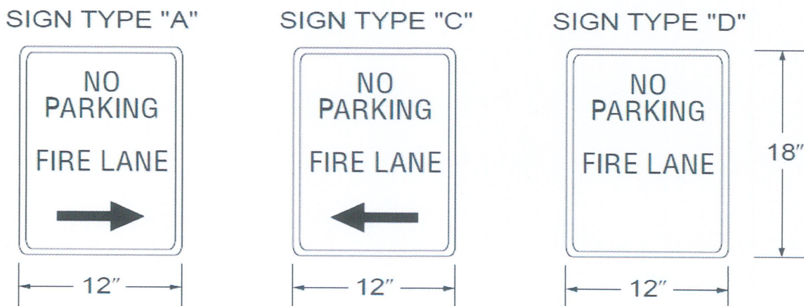
FIGURE D103.7 FIRE LANE SIGNS
